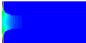
Fig. 24. (P4) Topology optimization plot of temperature response at iteration 159 using explicitly lumped convection matrices.
